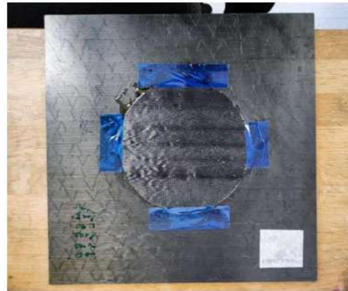
Figure 37: The patch prepared from carbon fiber/ 3R resin pre-preg
