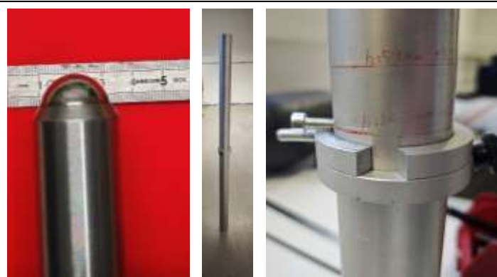
Figure 18 Detail of the impactor tip (left), free-fall apparatus used in the controlled energy tests (center) and impactor locking and releasing mechanism (right).
