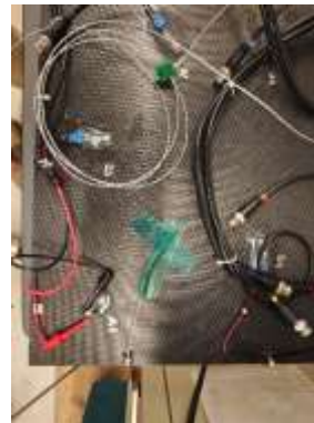
Figure 23. Detail of the temperature sensor placement on the CFRP plate surface (left) and climatic chamber used in the tests (right).
