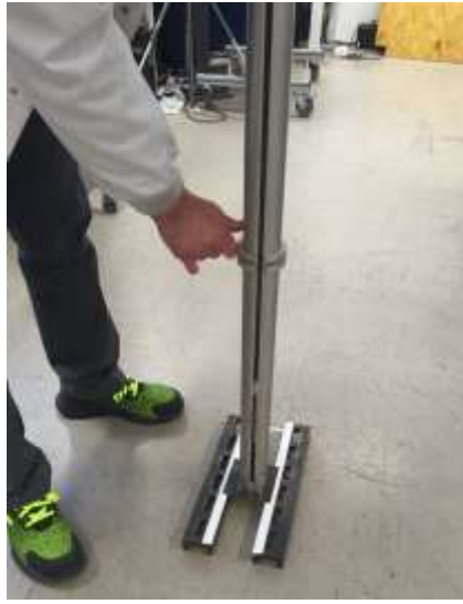
Figure 12. Drop weight impact testing at different energy levels (3, 6 and 9 Joules).
